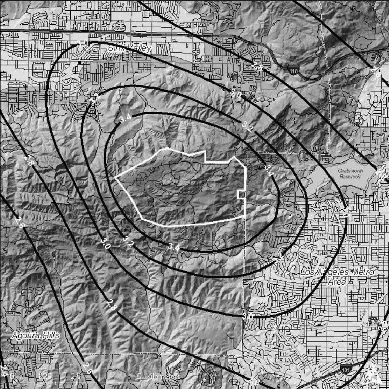
**Figure 3-14.** Contours of Locations of Highest Concentrations for the APTF Point Source Using the Best-Estimate Diurnal Emissions Profile
