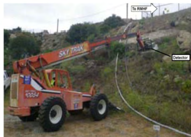
Enhanced Radiation Ground Scanner II (SkyTrak Telehandler) Scanning Hillside Behind RMHF
